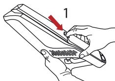
Pull out the battery in the direction of the arrow
