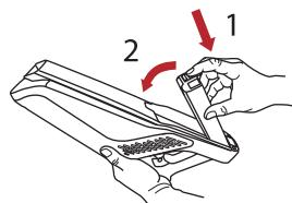
Hook the battery on the socket in the body
